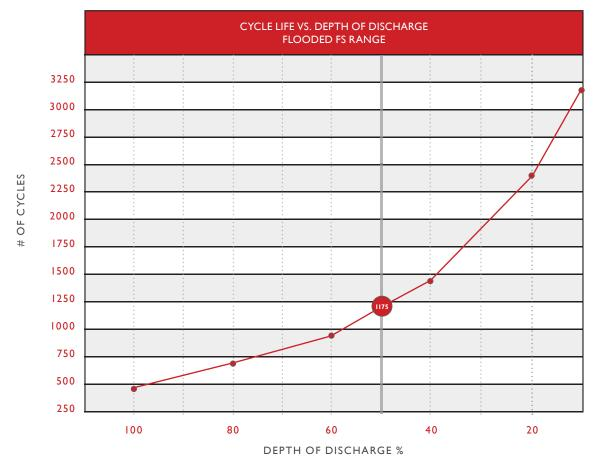
\*Cycle life may vary by application and is affected by frequency of cycling, operating temperature, depth of discharge (%DOD), adherence to manufacturer-recommended charging parameters and proper maintenance.
